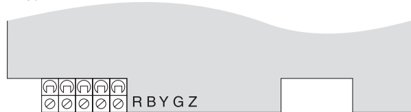
Keypad circuit board
